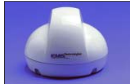
The PDT-100 is the satellite transceiver, antenna and 12-channel GPS. It has no moving parts.
