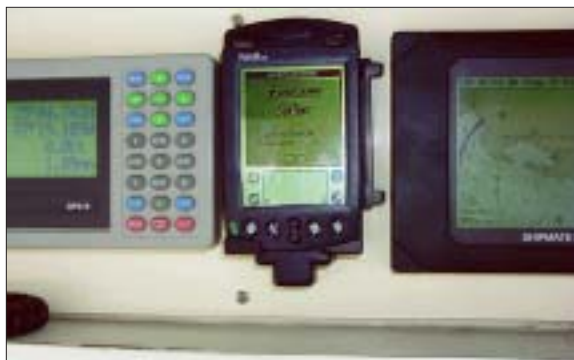
SeaTrac's cradle holds the Palm securely during transmission and reception yet allows easy removal for remote data entry. Backup units are inexpensive and readily available.
